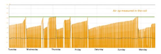
Pressure loss trend through the coil. The green line represents the threshold  $\Delta p$ , the blue curve represents the temperature sensor value.
