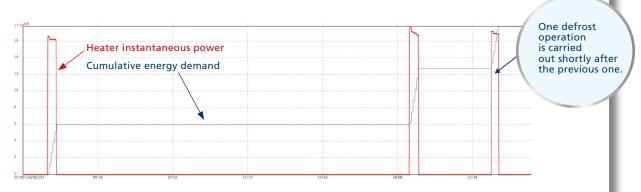
Trend over one day of power absorbed by the heaters. Around 20.45 there was an increase in the temperature in the cold room which caused the compressor to run continuously with the consequent need for a defrost shortly after.
